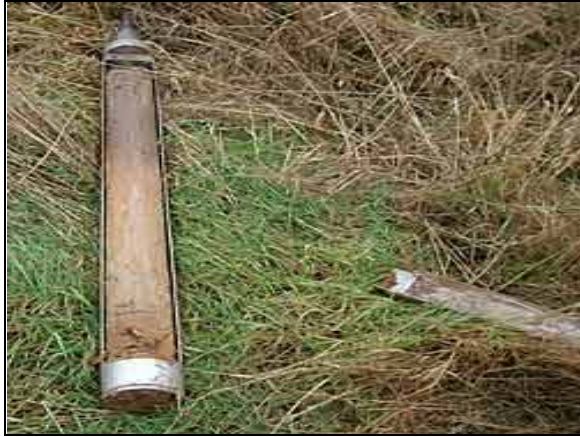
Figure C22: Soil core extracted for inspection and lab analysis to determine unconfined compression strength.
