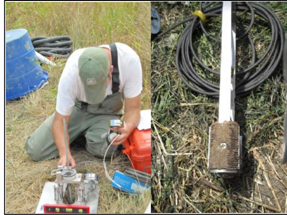
Figure C23: Iowa borehole shear test to make in situ measurements of bank geotechnical properties.
