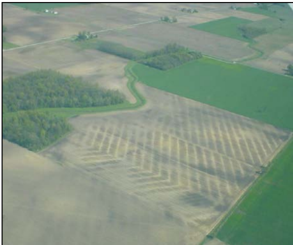
Figure 1: Aerial photograph of an agricultural field with subsurface drainage in Ohio. Location of subsurface laterals can be seen through differences in soil moisture.
